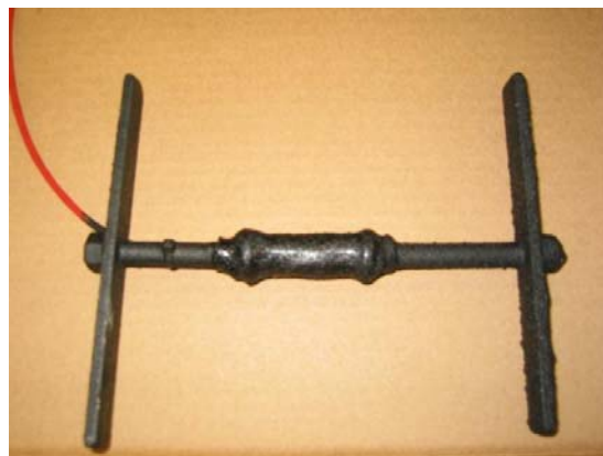
Figure 5.12: H-Type Asphalt strain gauges
