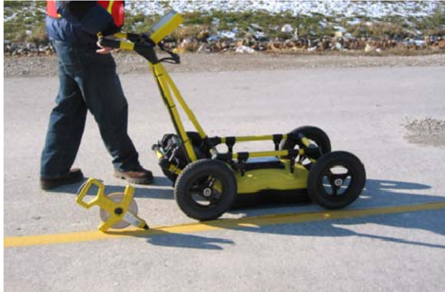
Figure 5.78: SmartCart ground penetration radar profiling system
