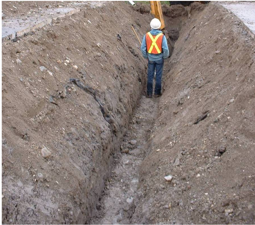
Figure 5.53: Excavated trench showing no sloughing prior to rainfall at test site
