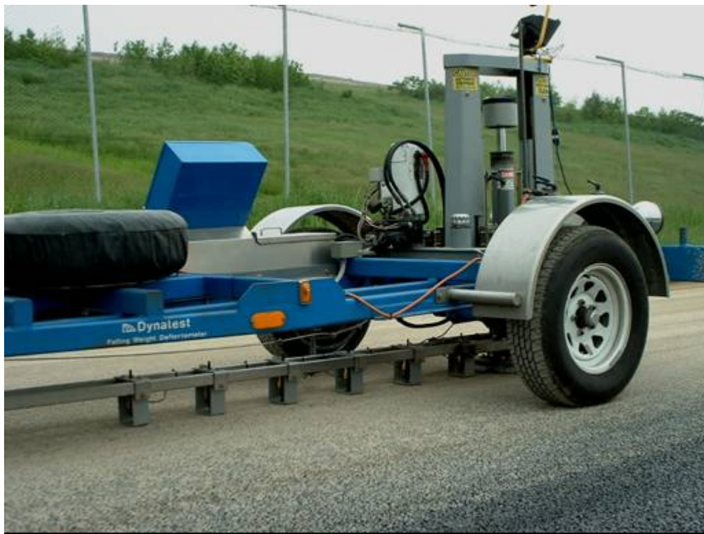
Figure 5.83: Dynatest model 8002-952 Falling Weight Deflectometer
