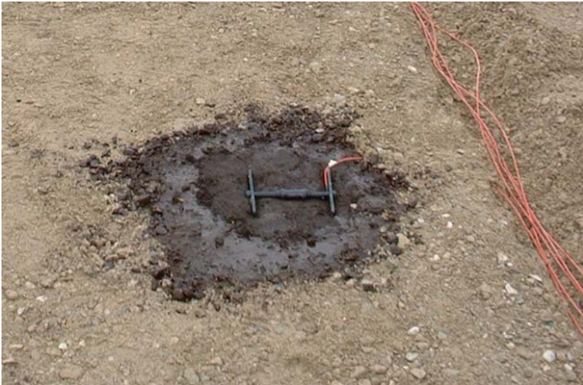
Figure 5.14: Asphalt strain gauge in sand-binder mixture
