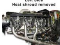
Heat shroud removed
