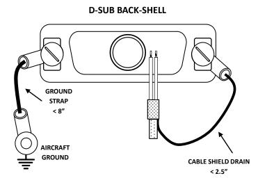
Figure 15 - Cable Shields and Ground Strap
