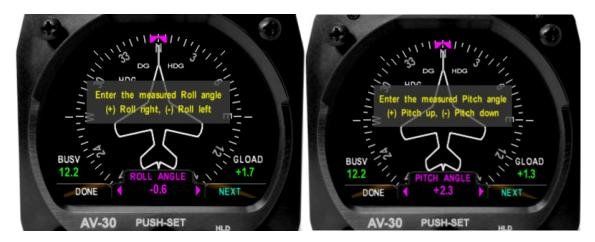
Once these values are committed, the AV-30 will calculate the differences in mounting angles for use in the heading solution. Once entered, changing these values without remeasurement of the AV-Mag angles will invalidate the installation calculation.
