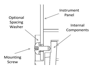
Figure 6 – Mounting Screw Depth Limits
