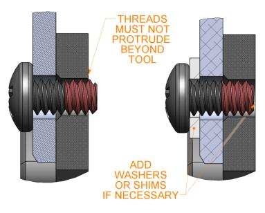
Figure 8 - Proper Screw Engagement Adjustment
