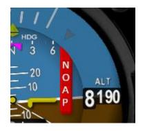
Follow the ground checkout procedure from your autopilot installation manual. In general, this involves setting the autopilot to heading mode and observing that the flight controls move in the correct direction as the heading bug is changed left and right of the current heading.
