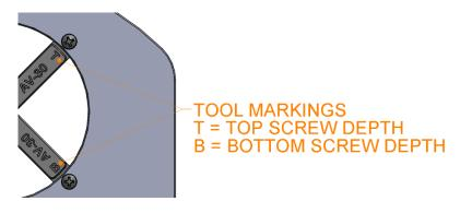
Figure 7 - Install tool used for Top and Bottom Screw Engagement Check
