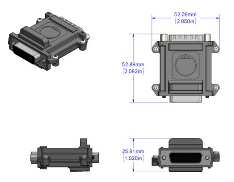
Figure 16 – AV-Link Mechanical Drawing
