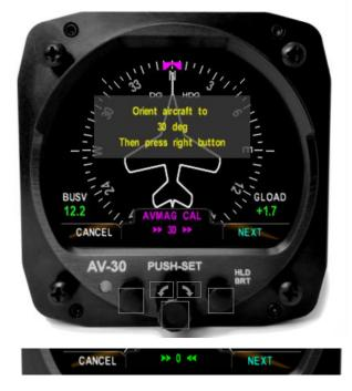
Figure 50 – AVMAG CAL Orientation Guide
