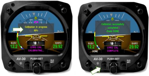
Figure 43 - Gyro Calibration Procedure
