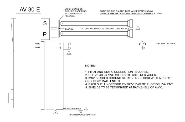
Figure 10 - Wiring Diagram – Required Connections
