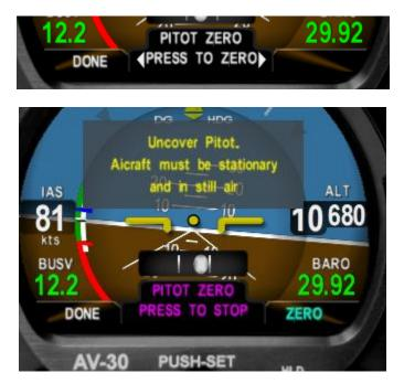
The PITOT ZERO function measures both the pitot and the static pressure sensor with identical air pressure conditions. Any difference in reading is saved and applied to subsequent airspeed calculations.
