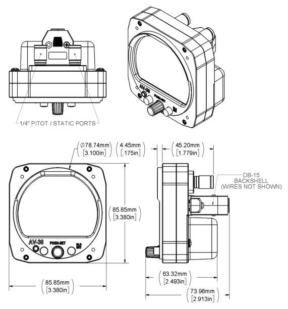
Figure 5 – Mechanical Drawing
