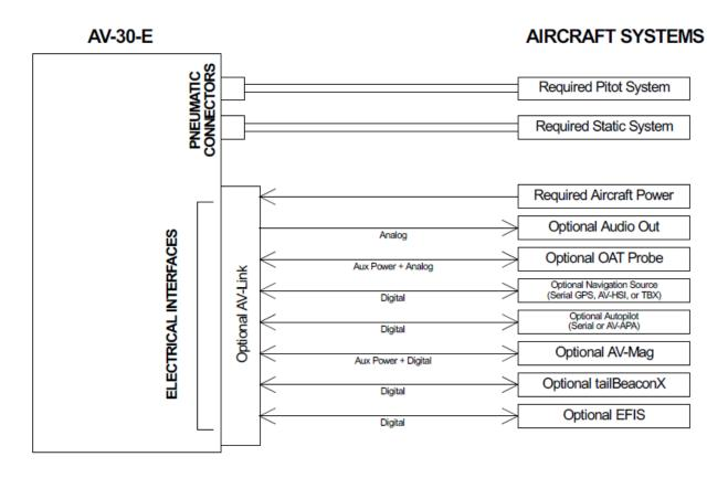
Figure 3 – AV-30 Aircraft Systems Interfaces – AI Mode
