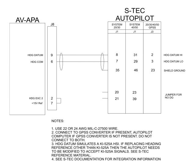
Figure 27 - AV-APA – S-TEC Interconnect Drawing
