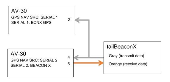
Figure 21 - Parallel tailBeaconX GPS Connections
