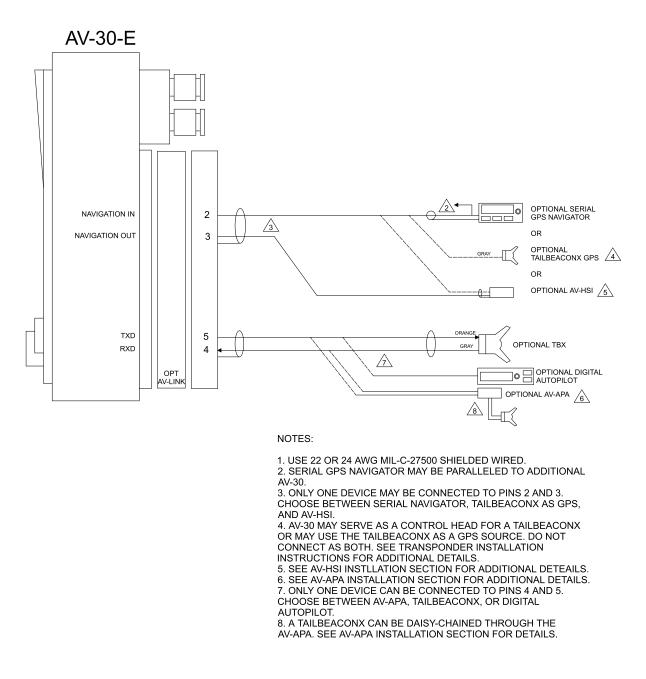
Figure 12 - Wiring Diagram – Optional Connections 2 of 2
