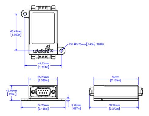
Figure 24 - AV-APA Mechanical Drawing
