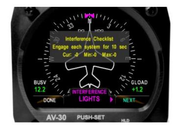
Use the rotary knob to step through each system in the checklist and monitor the magnetic field deviation value.
