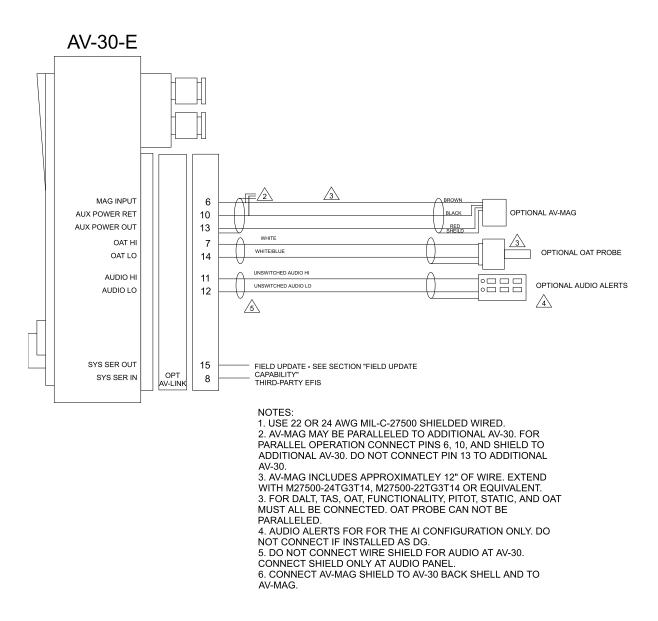
Figure 11 - Wiring Diagram – Optional Connections 1 of 2
