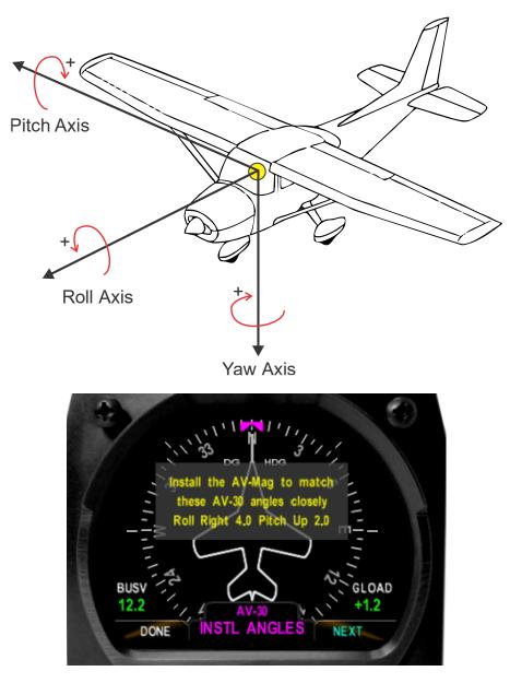
Adjust the AV-Mag mounting attitude to match that of the AV-30 as closely as possible. Simultaneously, the AV-Mag should be oriented as parallel to the line of flight as possible.
