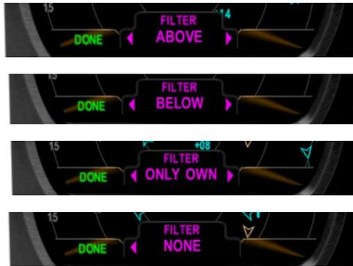
Figure 37 - Examples of Alternate Filter Values
