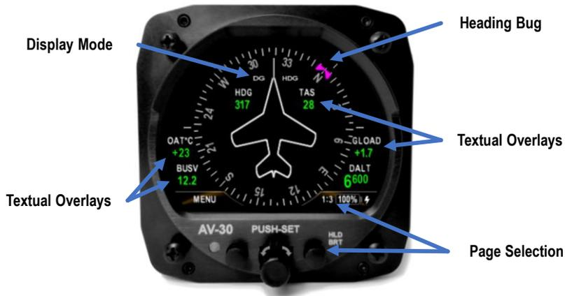
Figure 28 – Basic DG Mode User Interface
