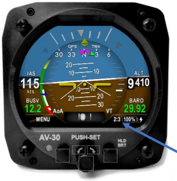
Figure 8 – Screen 2 of 3 showing GPS Ground Track, AoA, and Vertical Trend
