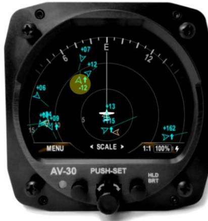
Figure 34 - Traffic Target Relative Altitude
