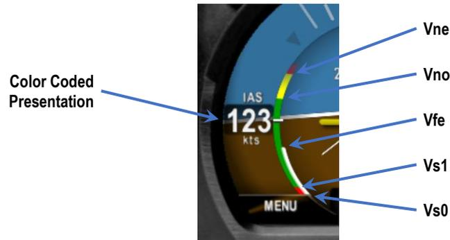
Figure 18 - AI Mode, V-Speed Limits
