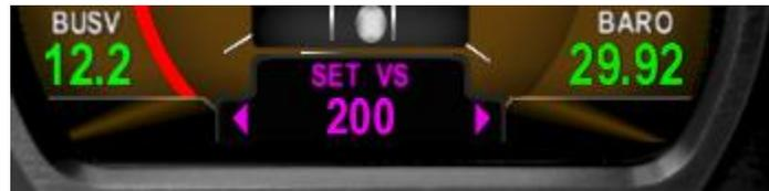
*Figure 52 Selected Vertical Speed entry*
