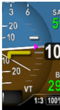
Figure 24 - AI Mode, Vertical Trend Indicator and SVS Bug
