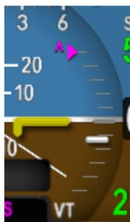
Figure 25 - SVS Bug value greater than scale
