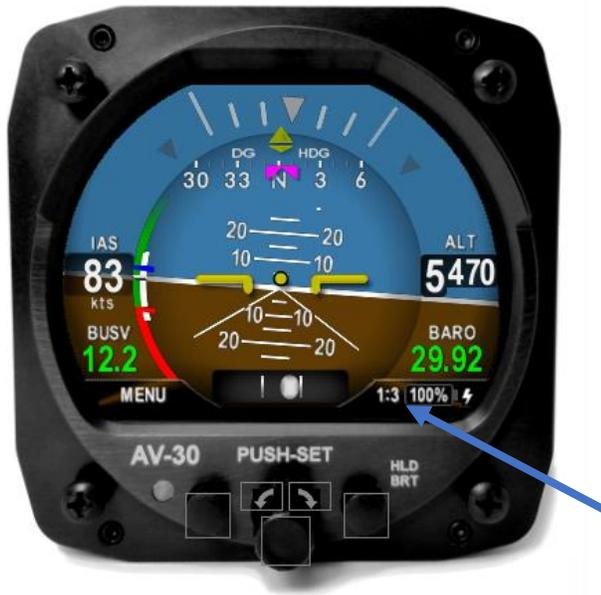
Figure 7 - Screen 1 of 3 showing Air Data and DG Heading
