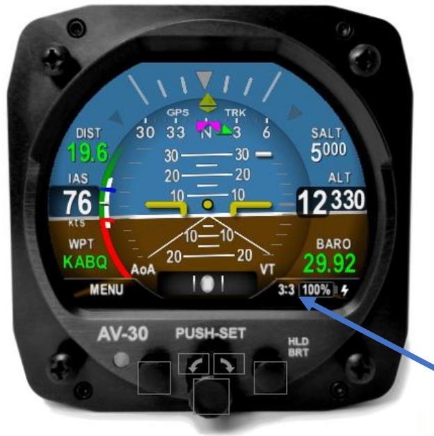
Figure 9 - Screen 3 of 3 showing Waypoint Data and SALT
