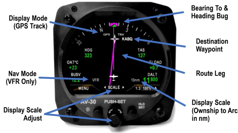
Figure 30 – GPS ARC Mode
