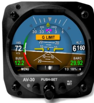
Figure 42 – Example of Alert Annunciator on Screen
