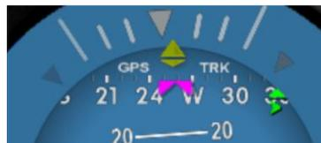
Figure 19 - AI Mode, Direction Indication, Bearing To Off-Screen
