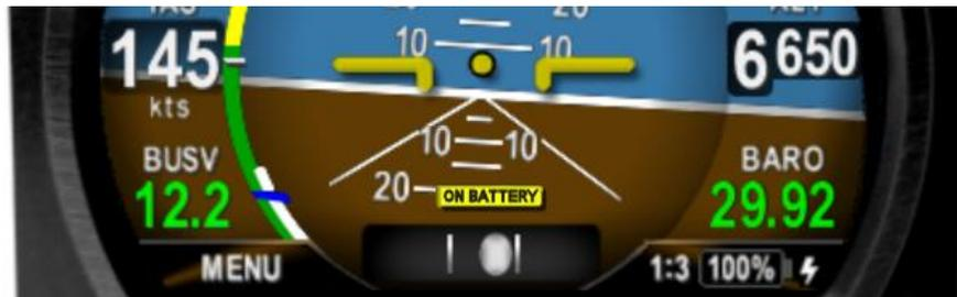
Figure 44 - On Battery Operation
