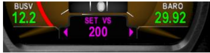
Figure 49 Selected Vertical Speed entry
