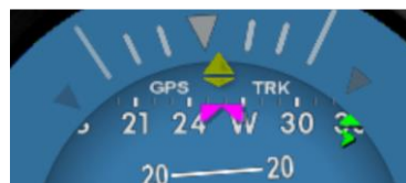
Figure 16 - AI Mode, Direction Indication, Bearing To Off-Screen
