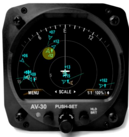
Figure 31 - Traffic Target Relative Altitude
