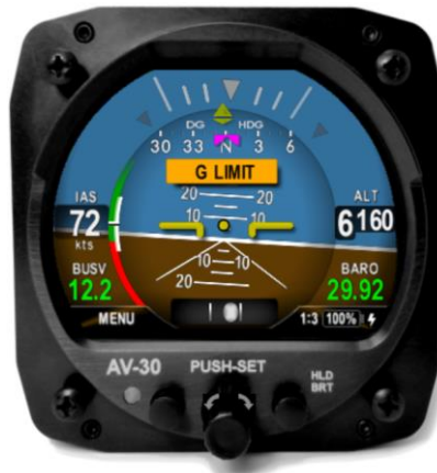
Figure 39 – Example of Alert Annunciator on Screen
