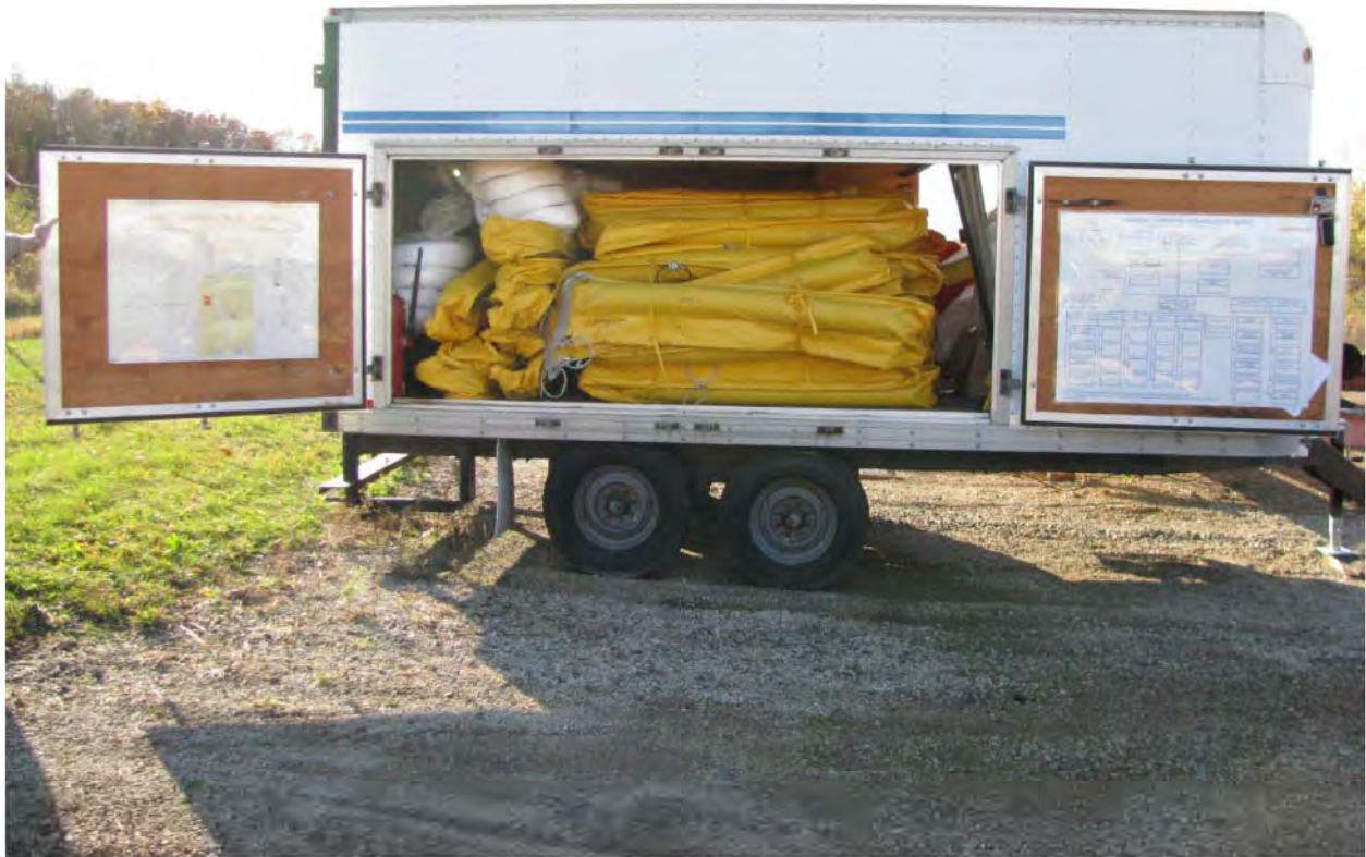
Figure 20. Enbridge PLM emergency response trailer containing the company's Tier 1 oil containment equipment, October 17, 2010.
