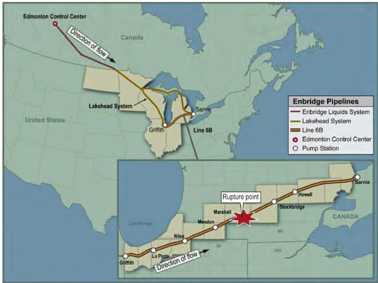
Figure 1. Enbridge’s Liquids System and the 1,900-mile Lakehead System (the U.S. portion). Inset shows Line 6B, the 293-mile extension from Griffith to Sarnia installed in 1969.
