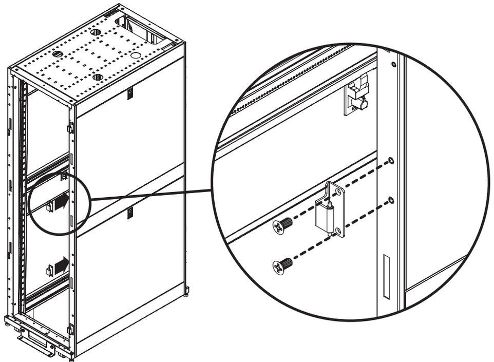
**For rear doors, move two hinge brackets so that all brackets are on the same side of the door frame.**
