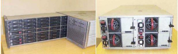
Figure 5: HP ExDS storage chassis, front and rear views Generic images courtesy Tim Reddin, HP Galway
