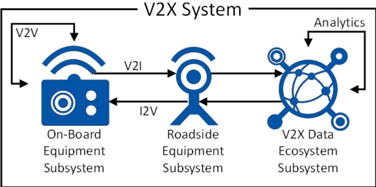
Figure 1 V2X System Components
