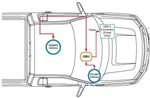
Figure 4 OBU Installation Diagram
