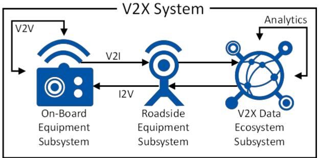
Figure 1 V2X System Components
