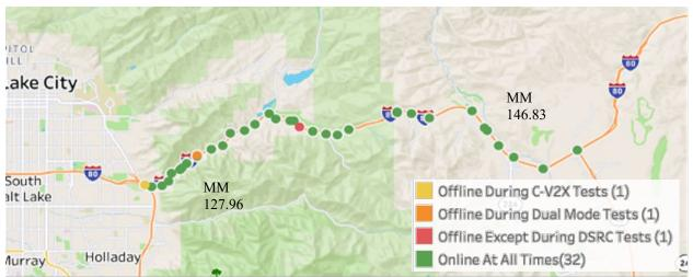
Figure 6 I-80 Test Location East of Salt Lake City (Note: Points show the 35 RSU locations on I-80)
