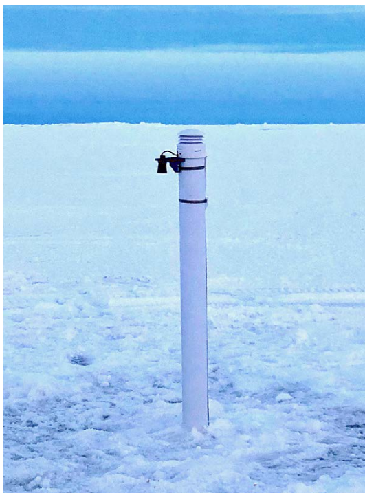
FIGURE 1. Photo of a Seasonal Ice Mass Balance (SIMB) buoy deployed in the Arctic. Photo credit: Ryleigh Moore
