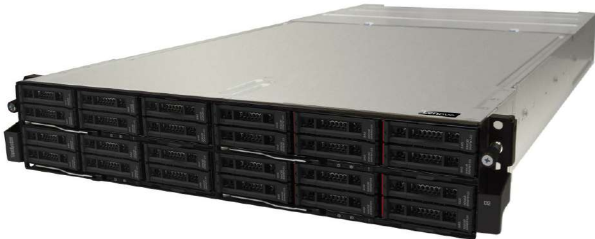
Figure 1. Four ThinkSystem SD530 servers installed in a D2 Enclosure
