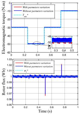
Fig. 7. Classical DTC strategy responses (test of robustness)
