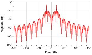
Fig. 3. Power spectrum of a BFSK signal (bit rate=20Kbps)
