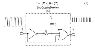
Fig. 11. Zero-crossing Detection
