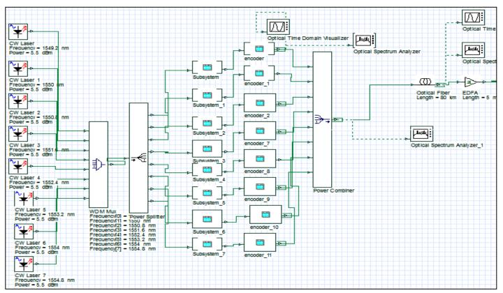
Fig. 7. OCDMA Transmitter block on Optisystem
