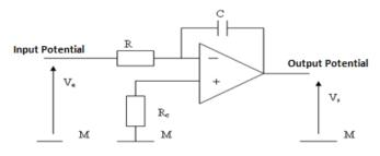
Fig. 4. Modeling of neuron outputs in the RSOM map by an electrical low-pass filter
