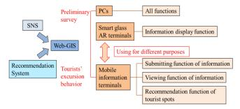
Fig. 1. System design of AR media GIS
