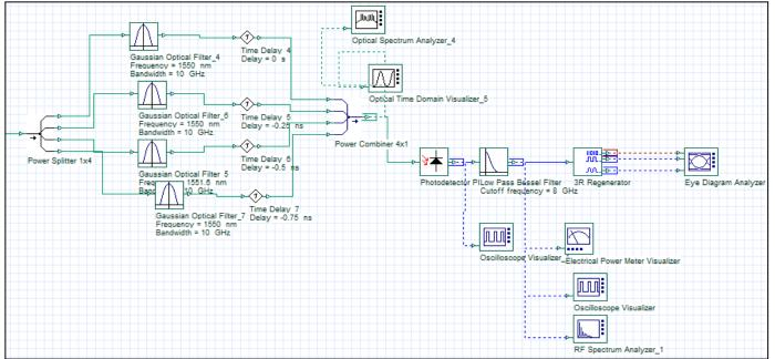
Fig. 9. OCDMA Receiver structure on Optisystem
