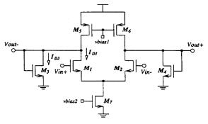
Fig. 9. Proposed limiting amplifier
