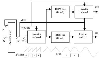
Fig. 5. Architecture of DDFS system
