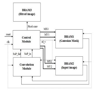
Fig. 3: Synchronous architecture of image filtering
