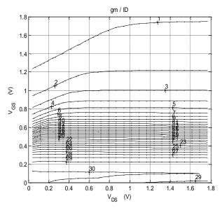
Fig. 9.  $\,$  gm/I\_D contours versus drain an gate voltages for 0.18  $\mu m$  gate length of NOMS transistor
