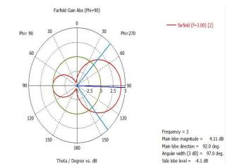
Fig. 9. 1D plot of Gain at Resonant Frequency Of 3.00 GHz
