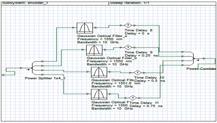
Fig. 8. Encoder Structure on Optisystem
