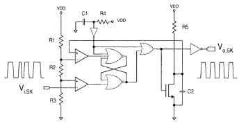
Fig. 12. The Shape keeping circuit
