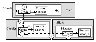
Fig. 5. FM representation of the crank-slider linkage system
