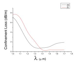
Fig. 5. Confinement loss plot according to wavelength
