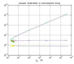
Fig. 13. Comaraison between W, A and  $V_{GS}$  predicted by EKV model (continuous lines) and its semi-empirical counterparts (crosses)
