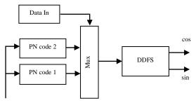
Fig. 4. Block diagram of the modulator
