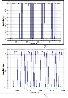
Fig. 11. Timing Diagram at 1Gbps for 1 user (a) Eye Diagram (b) Transmitted Signal (c) Received Signal
