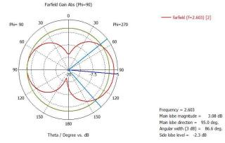
Fig. 6. 1D plot of Gain at Resonant Frequency 0f 2.603 GHz
