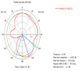
Fig. 12. 1D plot of Gain at Resonant Frequency of 6.58 GHZ
