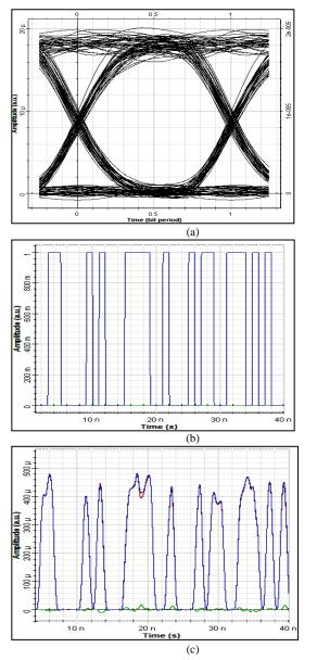
Fig. 13. Timing Diagram at 1Gbps for 8 users (a) Eye Diagram (b) Transmitted Signal (c) Received Signal
