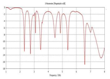
Fig. 11. Return loss of Bakelite
