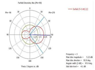
Fig. 10. 1D plot of Directivity at Resonant Frequency of 3.00 GHZ
