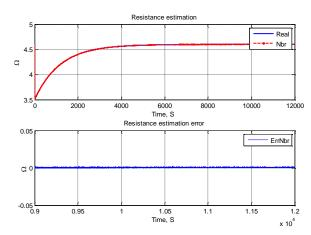
Fig. 10. Armature resistance estimation by ANN
