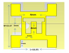
Fig. 4. Bottom View of Dual Fractal Patched Pi Antenna
