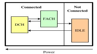
Fig. 2. Radio Resource Control Mechanism
