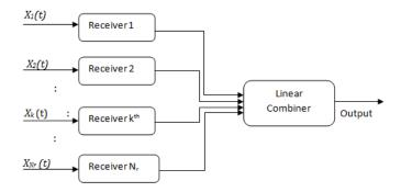
Fig. 3. Block diagram of Maximum ratio combining using  $N_{\rm r}\,$  receiving antenna
