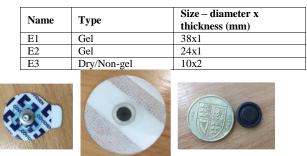
Fig. 4. Three ECG electrodes (from-left-to-right): E2, E1, and E3 (Table 1)
