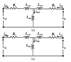
Fig. 1. Equivalent circuits of a DFIG: (a) on d-axis, (b) on q-axis
