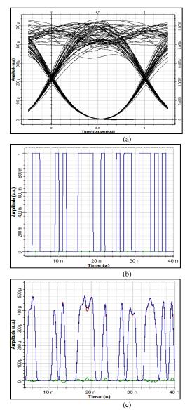
Fig. 14. Timing Diagram at 1Gbps for 12 users (a) Eye Diagram (b) Transmitted Signal (c) Received Signal
