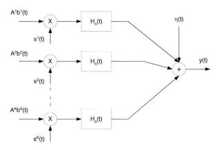
Fig. 1: Transmitter of a downlink CDMA system
