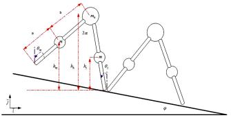
Fig. 2. Compass robot
