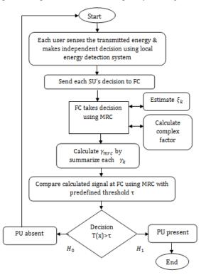
Fig. 4. Collaborative Energy detection using MRC
