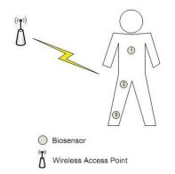
Fig. 1: Biosensors are implanted inside the body of a human to collect physiological measurements and transmit them over a wireless channel to an access point for further processing.
