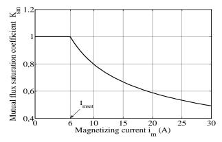
Fig. 3. Mutual flux saturation coefficient K<sub>sm</sub>
