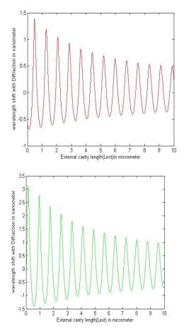
Fig. 7. Wavelength shift versus external cavity length is shown in (a) single ECTL formed by the external cavity comprised by curved micromirror and the front facet of the semiconductor (Red line) (b) Dual ECTL with two cavities formed by curved mirror in both sides. Radius of curvature of both cases a , b = 50 micrometer and reflectivity of mirror= .32 (green line)
