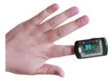
Fig. 6. Bluetooth finger PPG sensor
