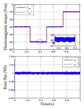
Fig. 6. DTC-HOSMC strategy responses (test of reference tracking)
