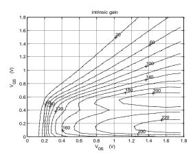
Fig. 10. Intrinsic gain contours versus drain and gate voltages
