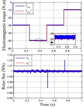
Fig. 5. Classical DTC strategy responses (reference tracking test)
