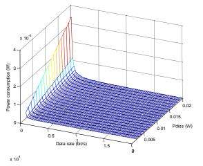
Fig. 2. Transmitter power consumption as a function of data rate and node power dissipation
