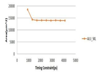
Figure 5: Scaling of Area of ALU-SKL with Timing Constraint
