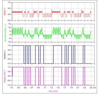
Fig. 17. Output signals of the demodulator
