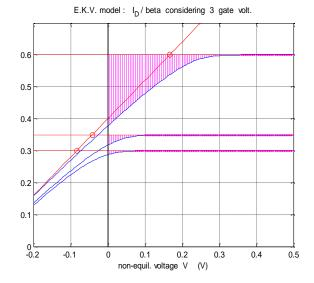
Fig. 1. Graphical illustration of drain current
