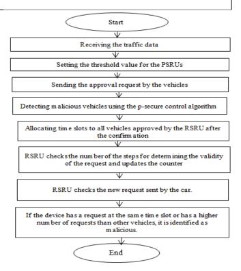
Fig. 4. Flowchart of the P-Secure approach
