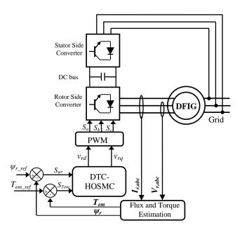
Fig. 2. Bloc diagram of HOSMC-DTC applied to the DFIG
