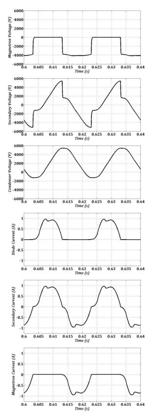
Fig. 4. B. Concordance of the theoretical waveforms, obtained by Matlab-Simulink, of currents and voltages (nominal mode)
