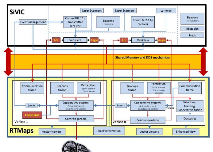
Fig. 3. CS simulation architecture's detailed functions in SiVIC-RTMaps™
