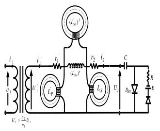
Fig. 3.  $\boldsymbol{\Pi}$  quadruple model of the transformer leakage referred to the secondary
