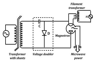
Fig. 2. Current power supply for one magnetron (Amperex technology)
