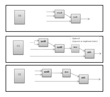
Fig. 11. The internal structure of the C0, C1, C2 building blocks.
