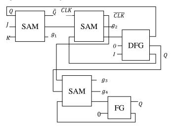
Fig. 15. Proposed Master Slave JK flip-flop with Q and  $\overline{Q}$  outputs
