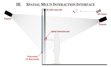
Fig. 1. The overall system layout.
