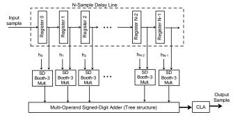
Fig. 4. Signed Digit FIR Filter [12]
