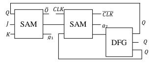
Fig. 14. Proposed Design of gated JK flip-flop with Q and Q outputs.
