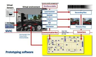
Fig. 1. General architecture of ADAS prototyping with SiVIC
