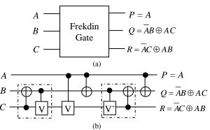
Fig. 4. (a) Block diagram of 3\*3 Frekdin gate and (b) Equivalent quantum representation
