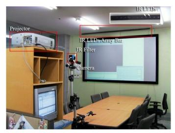
Fig. 8. The experimental environment for the proposed system.
