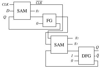
Fig. 17. Proposed design Master Slave D flip-flop with Q and Q outputs.
