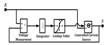
Fig. 6. Block Diagram of a non-linear inductance in Matlab-Simulink.
