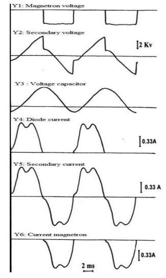
Fig. 8. Experimental waveforms of currents and voltages (nominal mode)
