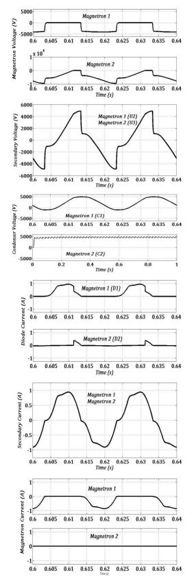
Fig. 11. Oscillograms of currents and voltages of the modeled circuit during the simulation in non linear regime with Matlab-Simulink code ( $M_2$  in failure)
