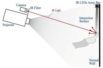
Fig. 3. Positions of the Projector and Camera.
