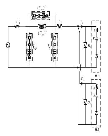
Fig. 7. Circuit of the new HV power supply for N = 2 magnetrons simulated using Matlab-Simulink code in nominal mode (non-linear regime)).
