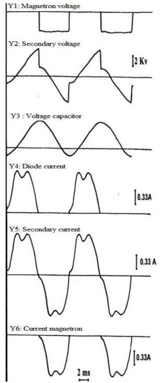
Fig. 4. A. Concordance of the experimental waveforms of currents and voltages (nominal mode)  $% \left( {{{\rm{C}}_{{\rm{c}}}}_{{\rm{c}}}} \right)$
