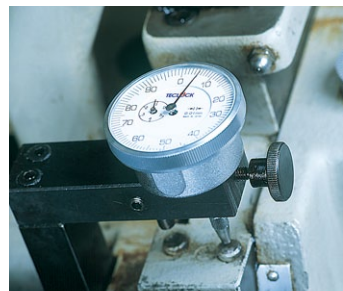
Displacement can be read from above.
