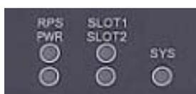
**Figure 3-5** Operating status LEDs of the A6602
