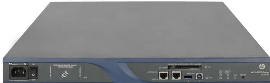
Figure 3-1 Front view of the A6602
