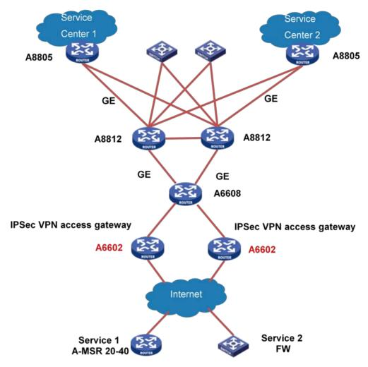
**Figure 5-1** A typical application network diagram with the A6602 acting as an IPSec VPN access gateway
