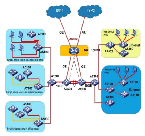
Figure 5-2 A typical NAT application network diagram with A6602s deployed
