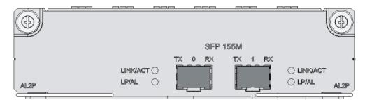
A JC495A (RT-HIM-AL2P) module is an OC-3/STM-1 (155 Mbps) Asynchronous Transfer Mode (ATM) interface module developed by HP. It provides two SFP interfaces and each interface is provided with two LEDs, which indicate interface running status and fault detecting status respectively.
