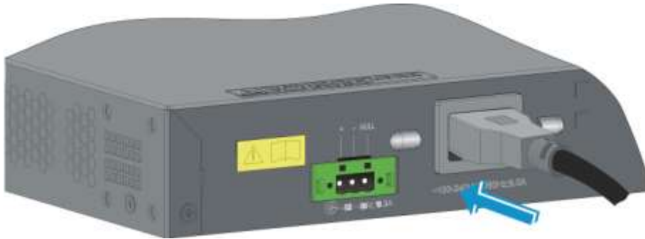
Figure 36 Connecting the AC power cord to the switch
