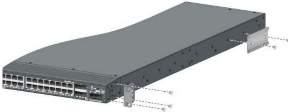
Figure 10 Attaching the front mounting brackets and the chassis rails to the chassis
