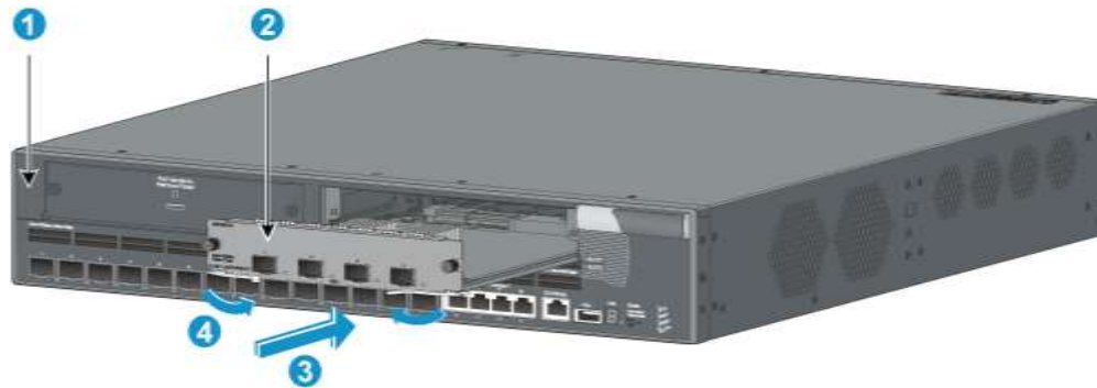
Figure 49 Installing an interface card
