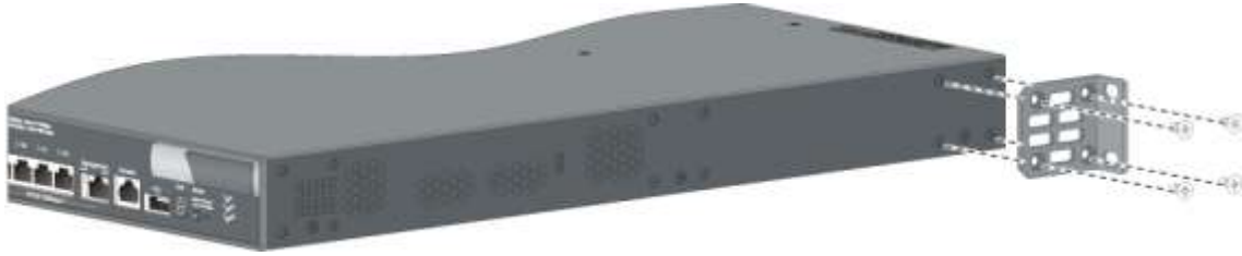
Figure 13 1U bracket rear mounting position
