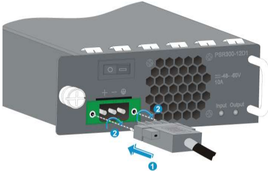
Figure 44 Connecting the PSR300-12D1
