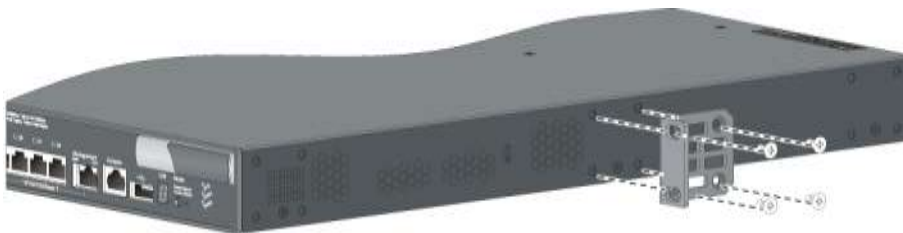
Figure 12 1U bracket mid-mounting position
