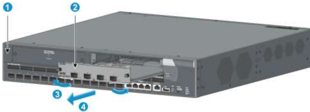
Figure 50 Removing an interface card
