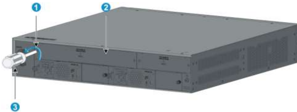
Figure 51 Removing the filler panel over the OAP card slot
