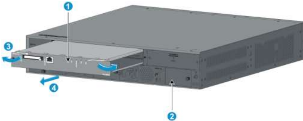
Figure 53 Removing the OAP card
