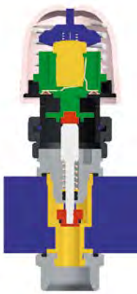
Type NC: Valve closed
