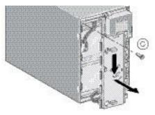
Remove the plastic protection cover in front of the battery (one screw).
