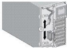
Disconnect the battery-module by separating the town connectors (never pull on the wires).
