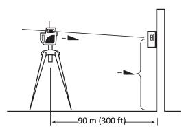
6. Measure the difference between the two marks. If they differ more than 5/16 in. (8 mm), you must calibrate the laser.
