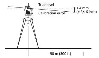
To check the horizontal calibration, you need a tripod with a %-11 threaded mount and a hand-held receiver. If you need to adjust the calibration, having another person to help saves time.
