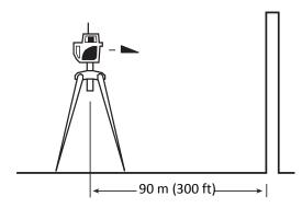
5. Raise/lower the receiver until you get an on-grade reading for the − ► axis. Using the on-grade marking notch as a reference, make a mark on the wall.
