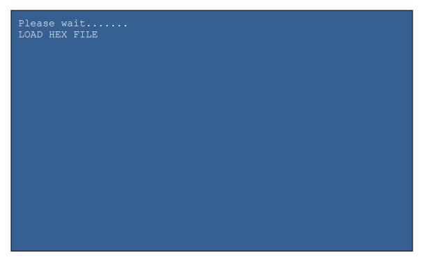
6. Within 40 seconds after *LOAD HEX FILE* appears, start sending the hex file using ASCII protocol (text file or raw binary) from the terminal application. When the file transfer completes, a checksum will be performed. If it is successful, Modemulator will be in AT command mode, with *OK* responses.
