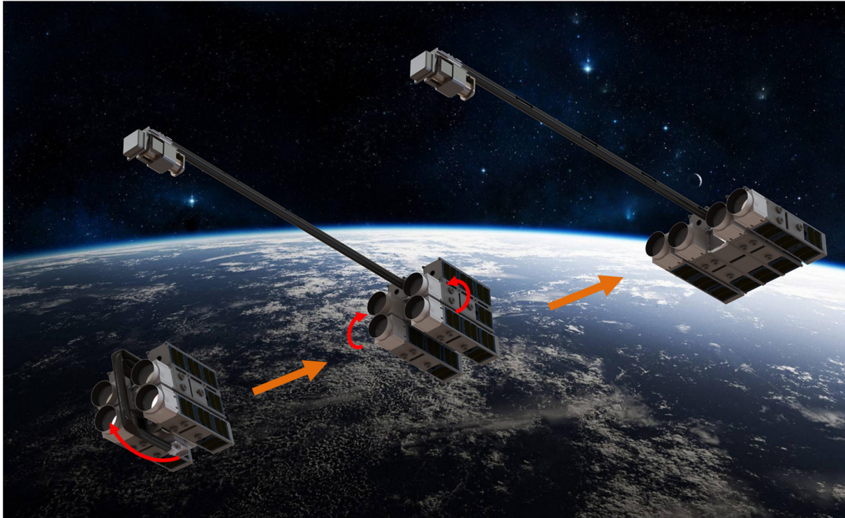
Fig. 2.4. Concept of the Autonomous Assembly of a Reconfigurable Space Telescope (AAReST) mission consisting of an arrangement of 10 cm diameter circular mirrors attached to a cluster of CubeSats. Image Credit: AAReST Team, California Institute of Technology ( http://www.pellegrino.caltech.edu/aarest1/ ).
