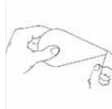
Label dispenses automatically when the liner is pulled from the front of the unit.
