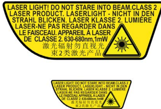
Figure 5 SE965 Protective Housing and Certificate Label
