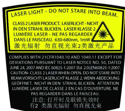
Figure 3 SE965 End-Cap Laser Warning Label
