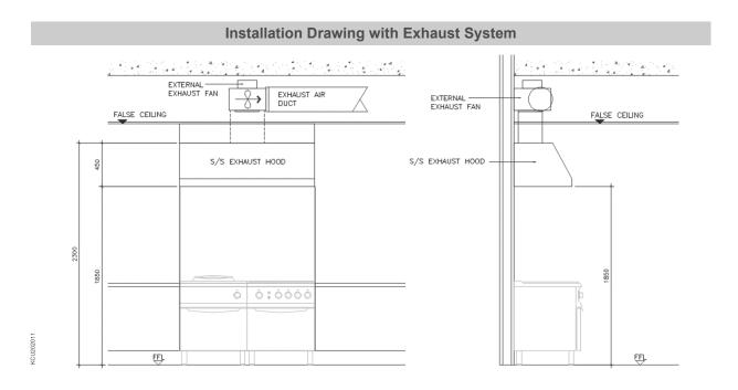
Remarks: The exhaust hood can be custom made according to customer's requirement.
