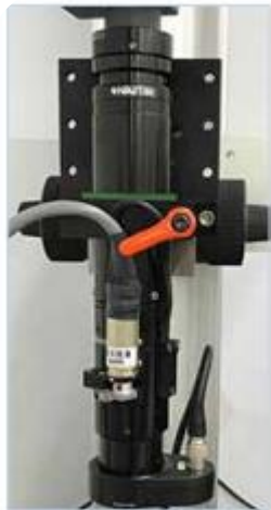
Optotune Module (Navitar 1-64805) with Zoom 6000 Motorized System
