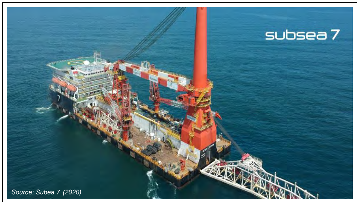
Photo 3.4. Subsea 7's Seven Champion S-lay pipeline installation vessel
