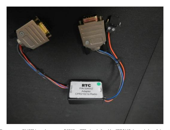
The converter 504552 is used to convert RS232 to TTL signals for older CPR2102 time switches. It is used in several designs, these modifications work for all of them.
