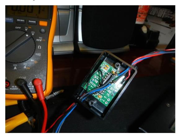
4. On the TTL connecter to the time switch you need to move the wire from Pin1 to Pin 9. This wire should be grey.
