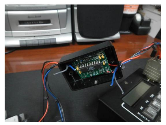
3. Solder the blue to the grey for both sides as seen below. Blue TTL to grey RS232, Grey TTL to Blue RS232. Once soldered insulate them from each other with either electricians tape or perhaps heat shrink tubing.
