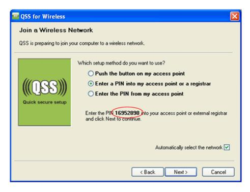
Figure 5-10 The QSS Configuration Screen of Wireless Adapter
