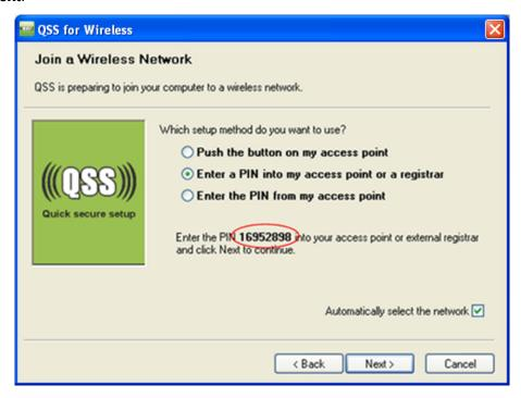
Figure 4-10 The QSS Configuration Screen of Wireless Adapter
