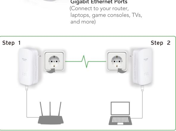
Note: Powerline adapters should be deployed on the same circuit and in set of two or more. The first, connected to the router and others located elsewhere to enable connectivity in those locations.
