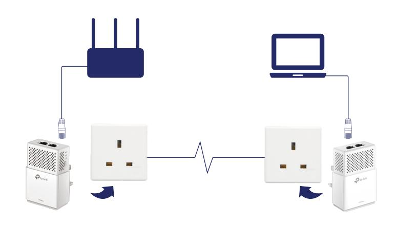
Powerline adapters and extenders must be deployed in a set of two or more.
