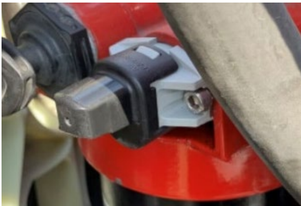
Figure 1: Fuel Heater Connector Cut
