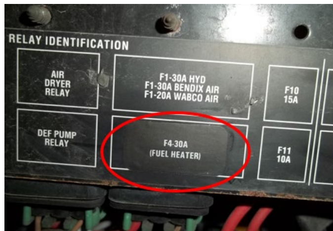
Figure 6: CE Bus 30A fuse sticker location with new sticker placed
