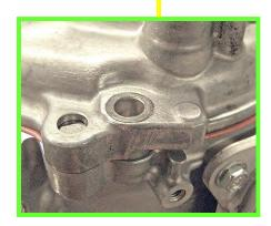
5. Align the primary pulley bearing retainer bolt holes with the bolt hole on the case as shown in Figure 5J.
