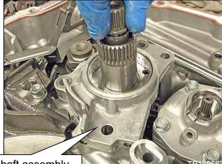
Input shaft assembly and the oil pump cover (dummy cover)
