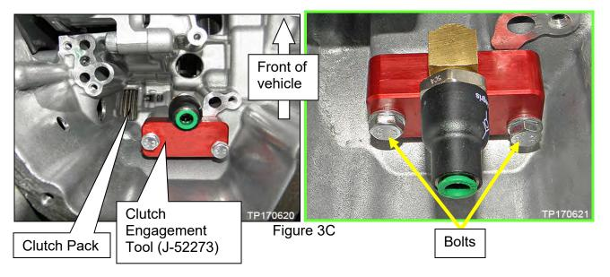
b. Connect the Hand pump from Evap Pressure Test Kit (J-42909) to the Clutch Engagement Tool (J-52273) and pump to 20 PSI.
