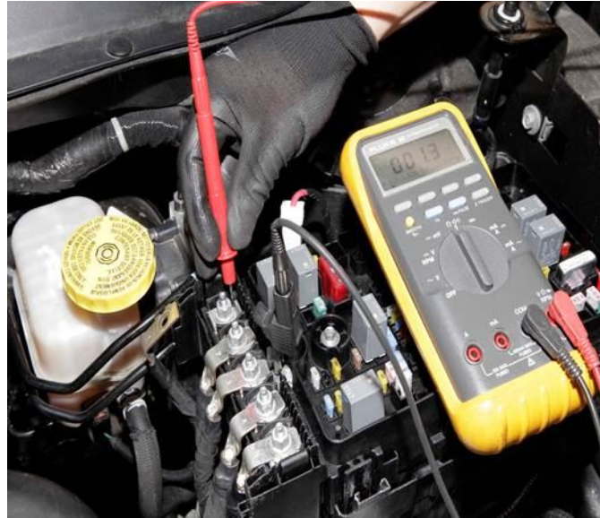
Fig. 13 Ohm Testing Fuses
