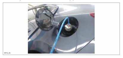
c. Plug the device in to turn it on and then open the pressure valve of the nitrogen supply to the device.
