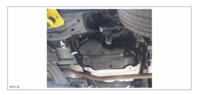
b. Disconnect the exhaust pipe.
