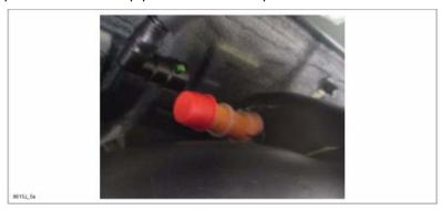
b. Connect the pressure output of the device to the filler pipe.
