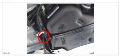
8. Disconnect the purge line from the fuel tank vent port using an unclipping tool.
