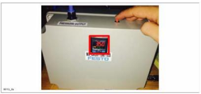
b. After 3.5 PSI is reached, keep holding down the red button for 10 more seconds to over fill the system, then release the red button (or push the rocker to off).
