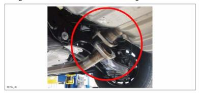
c. Loosen the the straps in order to lower the fuel tank.
