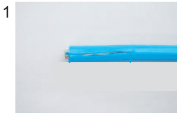
Expose inner vinyl sheath.
