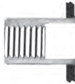
1. INSERT BLIND NUT INTO PREPARED HOLE.
