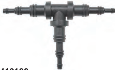
410100 3-Way Universal Tubing Connector For 1/8", 1/4" or 3/8" tubing. Break-Off Type Butyrate Plastic, For use with Vacuum & Windshield Washer Tubing Not For Use In Fuel Line. Box Qty. 5
