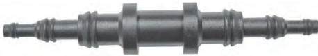
410105 Universal Tubing Connector For 1/8", 1/4" or 3/8" tubing. Break-Off Type, Butyrate Plastic For use with Vacuum & Windshield Washer Tubing Not For Use In Fuel Line. Box Qty. 10
