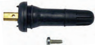
KX6-207A TPMS Rubber Snap In Valve 80psi max cold inflation pressure, Max Speed rating 115 MPH, T-10 Screw Torque 11.5in-lbs Box Qty. 1
