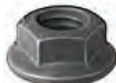
236005 11502722, 11502702 Black Finish Hex Flange Nut Thread: M5-0.8 Flange Dia.: 11.8mm Hex: 8mm Height: 5mm GM Box Qty. 50
