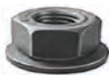
236004 N621900, N800466 Phosphate Free Spinning Washer Nut Thread: M4-0.7 Washer O.D.: 12mm Hex: 9mm Height: 4.5mm Box Qty. 50
