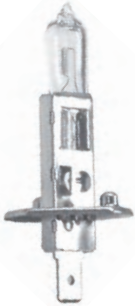
2294 9007 BULB High-Low Beam In Single Headlight Assemblies Box Qty. 1
