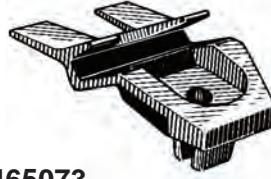
465073 75546-12010 Nylon Windshield Moulding Clip 20mm Wide, 40mm Long Fits Into 8mm Hole Box Qty. 10
