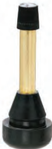
11413 High Pressure Snap-in Valve Ind. #: TR802HP Eff. Length: 2" Valve Hole Dia: .625" Max. Cold Inflation Pressure: 80 psi Not for use on tire rims that exceed .205" in thickness. Box Qty. 25
