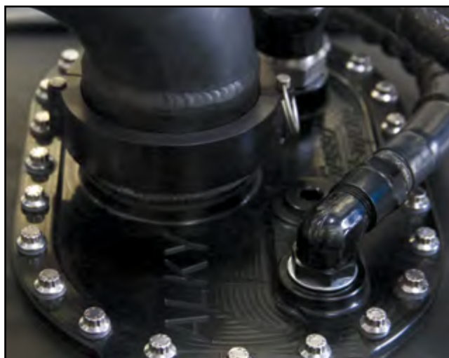
Maxwell Industries uses ARP weld bungs and stainless bolts on the Speed Demon fuel tank assembly.
