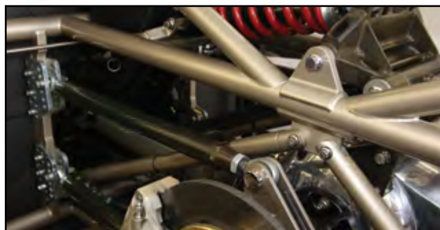
The world's fastest piston-engine car – Speed Demon – uses high strength ARP Stainless in the suspension and almost everywhere on the chassis.
