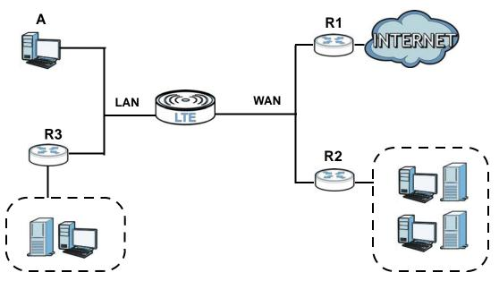
Figure 72 Example of Static Routing Topology
