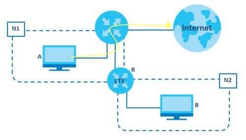
You need to specify a static routing rule on the Zyxel Device to specify **R** as the router in charge of forwarding traffic to **N2**. In this case, the Zyxel Device routes traffic from **A** to **R** and then **R** routes the traffic to **B**.
