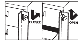
Locking Bars (used on 814-736 and 814-737, keep storage cabinet drawers securely shut.
