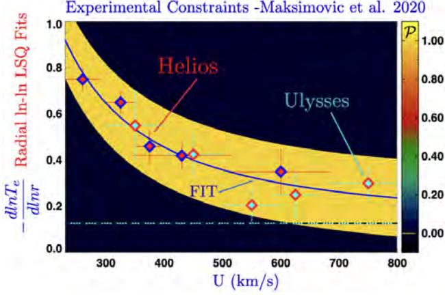
**Figure 13.** Empirical variations of  $\epsilon_{Te}(U)$  reported from Helios and Ulysses (crosses) versus solar wind speed  $U$ , with blue curve showing the fitted expression in Eq 27. Yellow band embraces essentially all error bars reported (Maksimovic et al. 2020) about the modeled profile.
