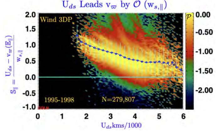
**Figure 25.** Wind strahl measured to have bulk speed  $U_{ds}$  displaced from the proton rest frame by parallel speeds at  $v_{\parallel} \geq v_{\varpi} + \mathcal{O}(w_{s\parallel})$ . This localizes the strahl as outside of the sphere of radius  $v = v_{\varpi}$  where coulomb collisions are dominant and produces nearly isotropic convecting Maxwellians. Cyan horizontal line corresponds to the strahl bulk velocity being at the outer radius of the collisionally dominant sphere.
