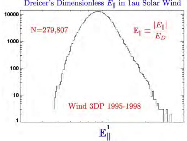
1181 **Figure 7.** Four year survey of direct measurements of Dreicer's dimensionless electric field,  $\mathbb{E}_{\parallel}$ , in the solar wind determined using a new technique developed for this paper demonstrating that  $\mathbb{E}_{\parallel}$  at temporal cadence of 96s is ubiquitously strong at 1au using all 279,807 readings obtained over 4 years between 1995-1998.
