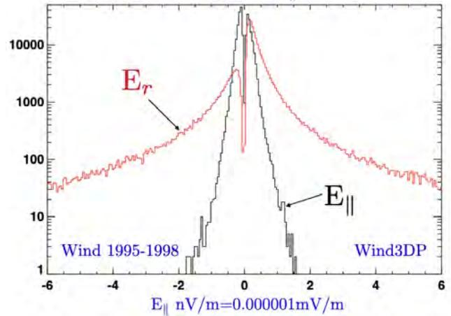
**Figure 11.** Four year distributions of  $E_{\parallel}$  (indicated in black) and the radial component of this parallel electric field  $E_r$  (in red) segregated by polarity relative to  $\hat{\mathbf{b}}$  and  $\hat{\mathbf{r}}$ .
