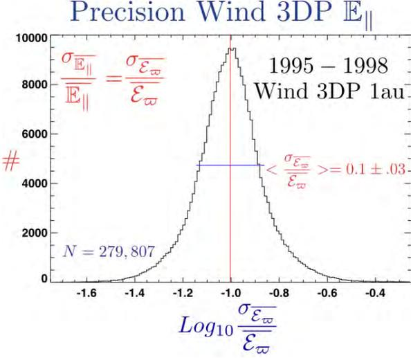
**Figure 12.** Histogram showing the average precision of the Wind determination of  $E_{\parallel}$  to be 10% using two separate estimates for each data determination via Eq 16.
