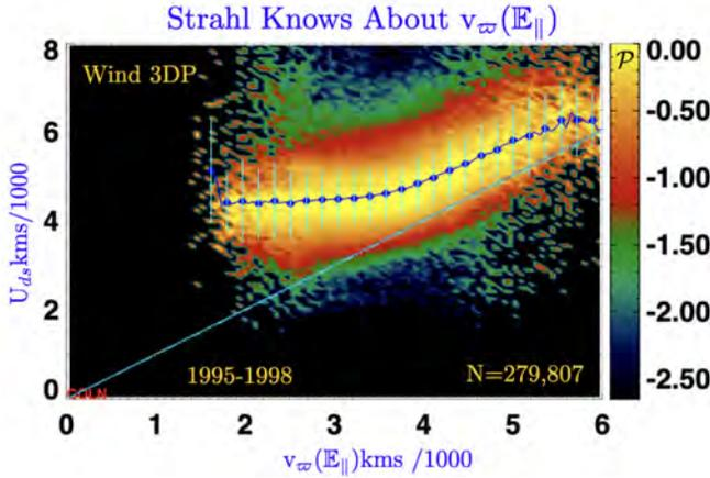
**Figure 24.** Overview of the size of strahl drift speed and the radius of the (red) spherical boundary in Fig 23 within which coulomb collisions are dominant. Inclined cyan line shows that the strahl bulk speed is invariable outside the sphere of coulomb dominance whose radius  $v_{\varpi}(\mathbb{E}_{\parallel})$  is numerically determined by the inventory of this paper that quantifies  $\mathbb{E}_{\parallel}$ .
