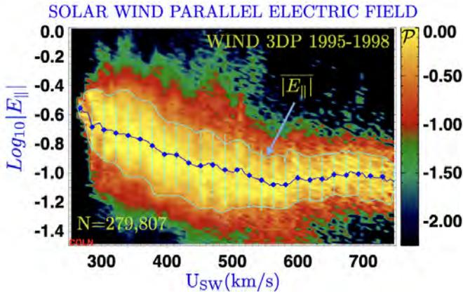
**Figure 10.** Bulk speed organization of probability of detection implied by Wind-SERM observations of  $\text{Log}|E_{\parallel}(\text{nV/m})|(U)$ . The superposed blue connect-o-dot curve joins the 80 vertical column averages. This curve (with column variances indicated by the cyan flags) show the bulk speed trend of the column mean. For reference the cyan contour is the locus of probability  $e^{-1}$  throughout the 2-D histogram.
