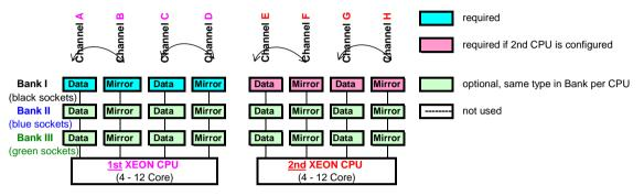
Mirrored Channel Mode requires identical modules on channel A,B, C, D (1st CPU) or channel E, F, G and H (2nd CPU) 50% of the capacity is used for the mirror => the available memory for applications is only half of the installed memory If this mode is used, a multiple of 4 identical modules has to be ordered.
