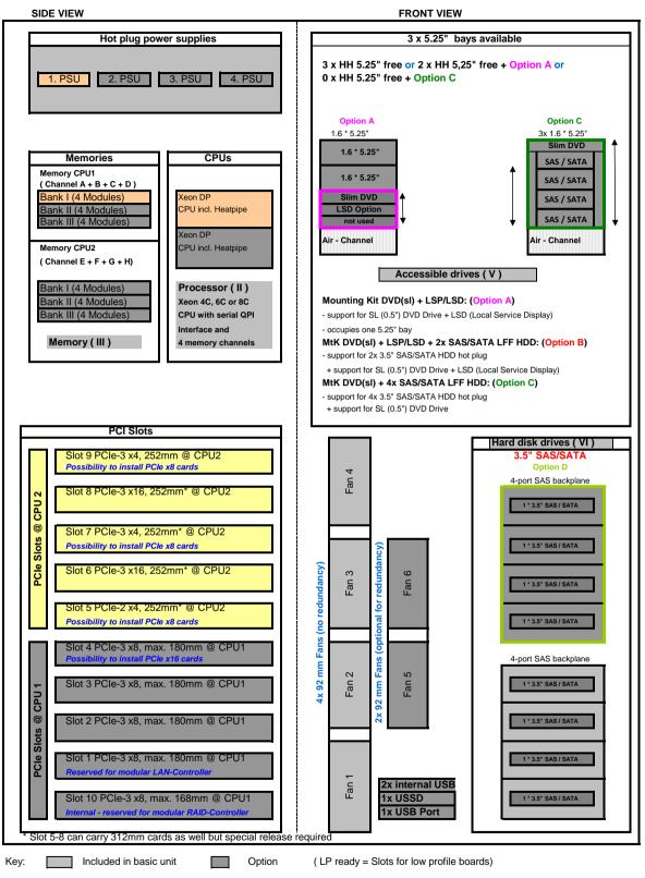
One CPU, one memory per CPU and one PSU has to be selected for an orderable basic unit.
