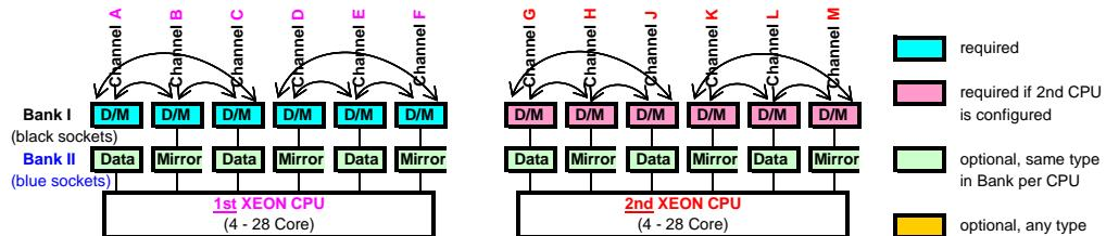
Mirrored Channel Mode requires identical modules on channel A, B, C, D, E, F (1st CPU) or channel G, H, J, K, L and M (2nd CPU) 50% of the capacity is used for the mirror => the available memory for applications is only half of the installed memory. If this mode is used, a multiple of 6 identical modules has to be ordered.
