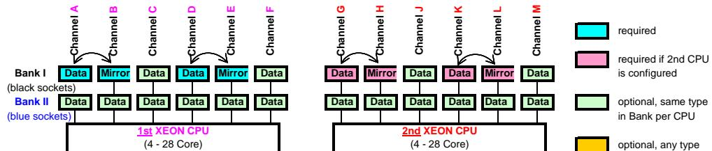
Mirrored Channel Mode (4 DIMMs per CPU) requires identical modules on channel A, B, D & E (1st CPU) or channel G, H, K & L (2nd CPU) 50% of the capacity is used for the mirror => the available memory for applications is only half of the installed memory. If this mode is used, a multiple of 4 identical modules has to be ordered.
