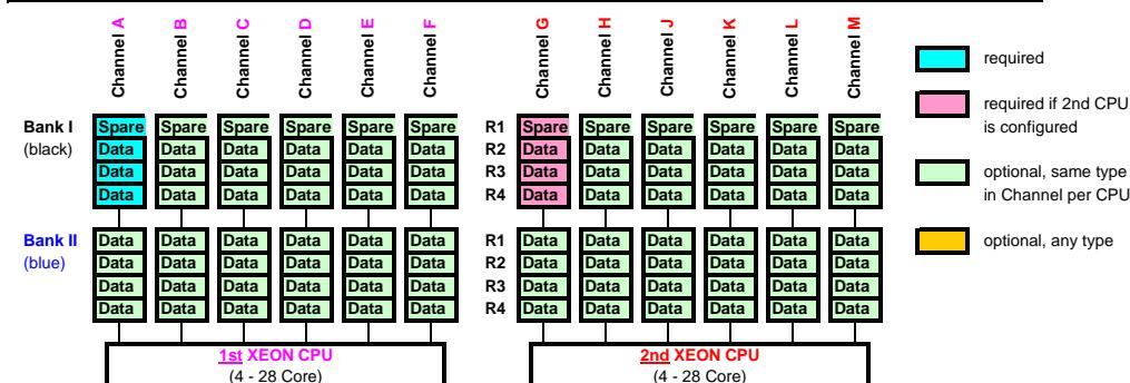
Rank Sparng Mode requires identical modules (same capacity and technology) within the same channel. The available memory for applications will vary depending on configuration. Please refer to the spreadsheet above "Effective Memory capacity with active Rank Sparng Mode". Population rule for Rank sparing mode is to achieve max. available memory, e.g. 4 DIMMs will be spread across two channels, each with 2DPC
