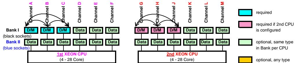
Mirrored Channel Mode (3 DIMMs per CPU) requires identical modules on channel A, B & C (1st CPU) or channel G, H & J (2nd CPU) 50% of the capacity is used for the mirror => the available memory for applications is only half of the installed memory. If this mode is used, a multiple of 3 identical modules has to be ordered.
