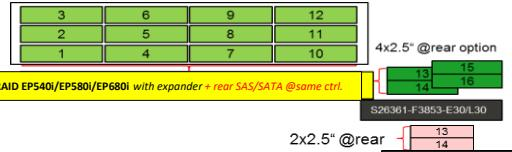
**Basic unit SFF optimized for Flash Applications (PCIe SSD)**
