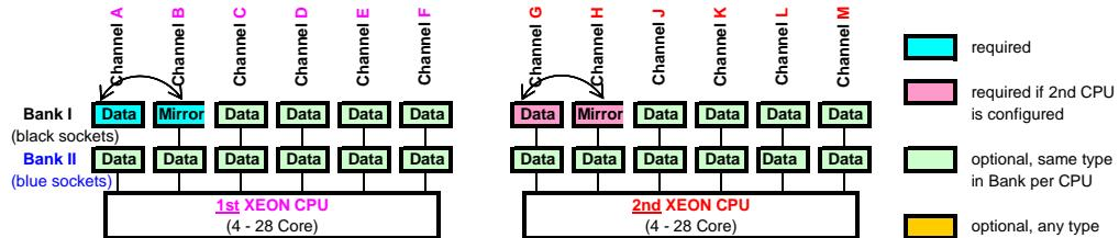
Mirrored Channel Mode (2 DIMMs per CPU) requires identical modules on channel A & B (1st CPU) or channel G & H (2nd CPU) 50% of the capacity is used for the mirror => the available memory for applications is only half of the installed memory. If this mode is used, a multiple of 2 identical modules has to be ordered.
