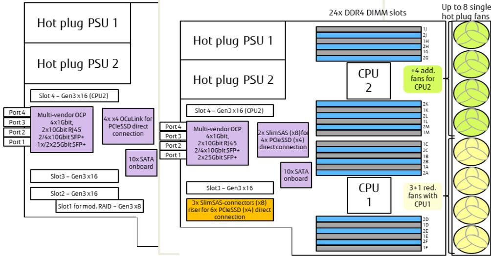
**PRIMERGY RX2530 M5 rear view with PSU, PCIe slots and dynamic LoM**
