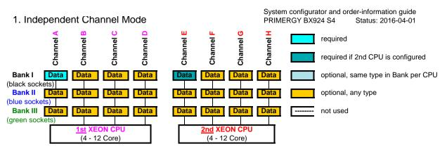
Independent Channel Mode allows all channels to be populated in any order Can run with differently rated DIMMs and use the settings of the slowest DIMM installed in the system
