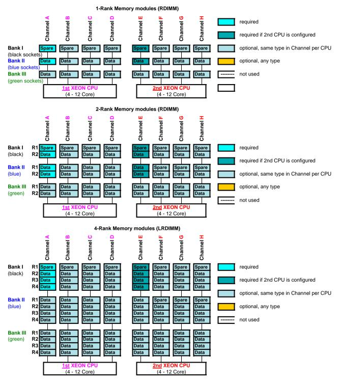
Rank Sparing Mode requires identical modules (same capacity and technology) within the same channel. The available memory for applications will vary depending on configuration. Please refer to the spreadsheet above "Effective Memory capacity with active Rank Sparing Mode". Population rule for Rank sparing mode is to achieve max. available memory, e.g. 6 DIMMs will be spread across two channels, each with 3DPC
