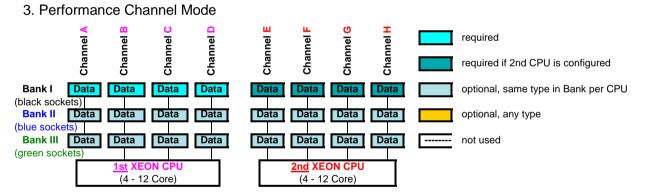
Performance Channel Mode requires identical modules on all channels of each Bank per CPU. If this mode is used, a multiple of 4 identical modules has to be ordered.
