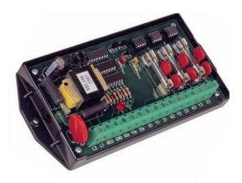
voltage of +13VDC is available on the "Yin" and "Zin" inputs, and is "pulled up." "Kin" is the common return. The SPR-3 may be used with meters having electromechanical output contacts (relays), or high or low voltage semiconductor outputs.
