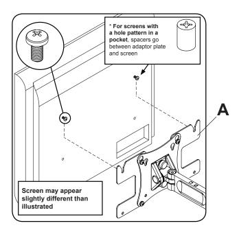
Depending on the make of your screen, insert one M4 x 10mm, M5 x 10mm or M6 x 10mm screw through each bottom hole of the adaptor plate ( $\bf A$ ) as shown below.
