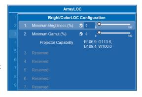
If the projector falls below the minimum, the projector operates at its current brightness and gamut. Changes will not be made.
