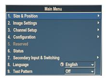
With a function menu displayed, enter a menu option number for any numbered option, or use the UP/DOWN arrow key to highlight the desired option and then press ENTER.
