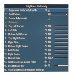
projector response time while adjusting settings. To disable the **Brightness Uniformity** function, delete the **Brightness Uniformity Enable** checkmark.
